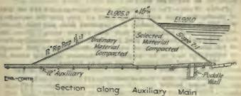
Fig. 28.—Sections of Earth Dam.
